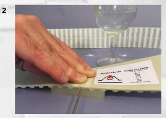
Begin to thread the pin by using an electric screwdriver and water (using as lubricant), to help the threading. For a correct alignment, use the plate/piece of belt furnished, like photo.
