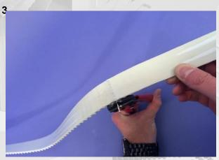
Cut the pin the nearest of the edge of the belt
