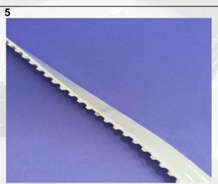
Check that the pin doesn't exceed any edge of the belt.
