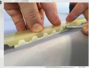
When the pin is completely inserted in the belt, break the pin at the precut area.
