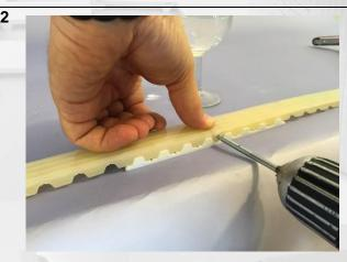
Begin to thread the pin by using an electric screwdriver and water (using as lubricant), to help the threading. For a correct alignment, use the furnished piece of belt, like photo.
