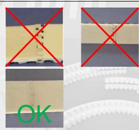
Cables are in contact with the pin; be careful to prevent any cables damages during the installation
