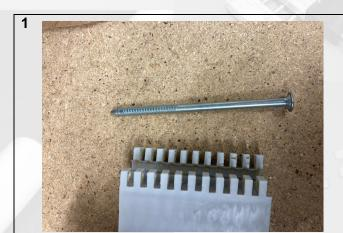
Align the teeth. Teeth must be correctly aligned to avoid any cables damage during pin threading. Misalignment of teeth or the using of a non-chamfered pin can damage the belts cables during the installation
